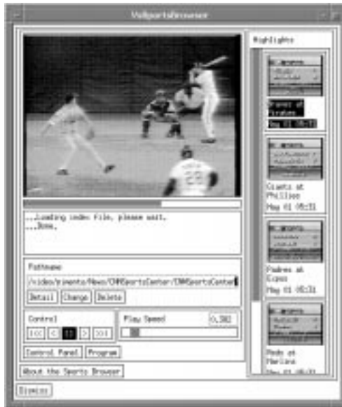
Figure 1.2: The Sports Highlight Browser , an application that supports content-based retrieval of video segments from a television program using video analysis.
